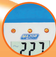
Correct Wiring Indication
