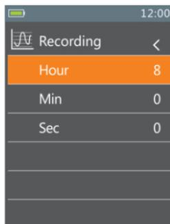
Setting of recording duration from 1min to 9h:59min.
