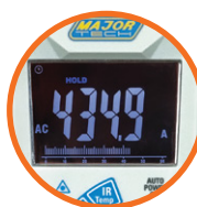
6000 Count Backlit Negative Colour Display
