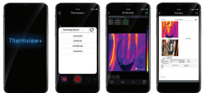
Built-in Infrared Thermal Imager offers you non invasive measurements of potential hot spots. These images can be transferred via Bluetooth to a Smartphone for analysis. Simply turn on the bluetooth of the smartphone. Press the Thermview+ icon and enter into the home interface, then press the Connect Device icon and the bluetooth device name will appear. Touch the device name listed in Bluetooth devices list to connect to the device.
