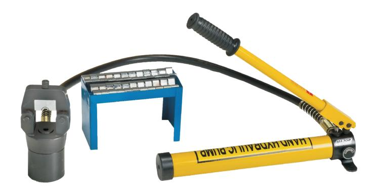
The Hydraulic Crimping Tool Set offers a maximum crimping force of 22T and a 22mm<sup>2</sup> stroke, ensuring precise and efficient crimping. It covers a wide crimping range from 16mm<sup>2</sup> to 400mm<sup>2</sup>, using a hexagonal crimping type for accuracy. The set includes crimping dies for various copper conductor sizes, from 16mm<sup>2</sup> to 400mm<sup>2</sup>. For a reliable and comprehensive hydraulic crimping tool set, trust this product to handle various crimping tasks with ease.
