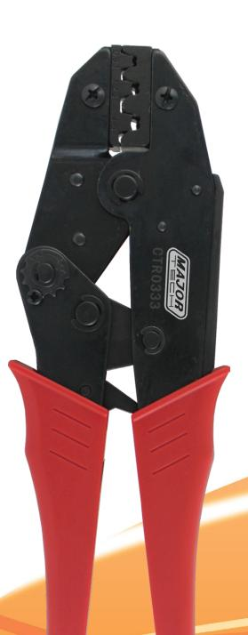
Major Tech's 1.5mm-6mm² Crimping Tool is designed for automotive and white goods terminals, with compatibility for sizes 1.5mm<sup>2</sup>, 2.5mm<sup>2</sup>, and 6.0mm<sup>2</sup>. It offers automatic release with manual override for precise and efficient crimping. The tool's professional-quality, drop-forged jaws are suitable for non-insulated terminals. With a length of 225mm2, it's a reliable addition to your toolkit for various crimping tasks.
