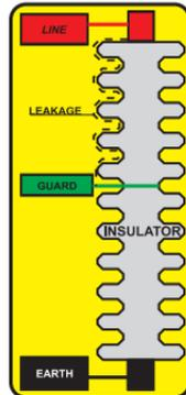
Resistance due to contamination can be very low and lower the total resistance. Cleaning periodically can also reduce system power consumption.
