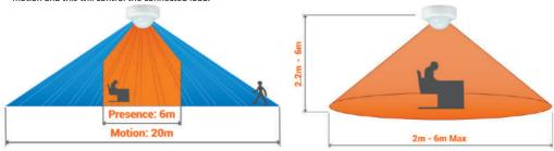
Note: PIR Presence Sensors, also known as PIR Occupancy Sensors, reply on line-of-sight and look for changes in heat in the detection area - if you have minimal movements or move slightly, the PIR sensor will pick up these changes and know you are there. These occupancy sensing methods help ensure that the lights or other electrical equipment systems only run when needed, saving energy without omitting you in the room.
