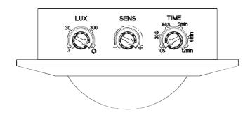
**NOTE:** The high-frequency output of the HF sensor is <0.2mW that is just one 5000<sup>th</sup> of the transmission power off a mobile phone or the output of a microwave oven. Keep away from children.
