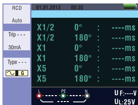
RCD Standby Screen
