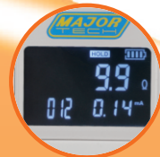
Black LCD that Simultaneously Displays Resistance & Current
