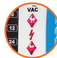
Live Warning Only, Danger
